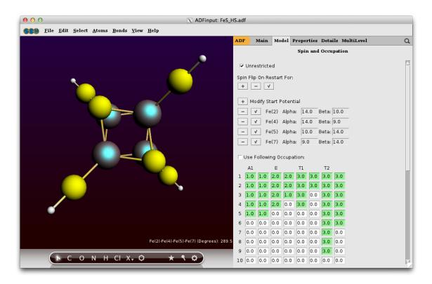
For the spin-up  $\text{Fe}^{3+}$ , S = 5/2, the alpha and beta numbers would be 14 and 9, correspondingly, and for the spin-up  $\text{Fe}^{2+}$ , S = 2, these numbers are 14 and 10. For the spin-down Fe sites, alpha and beta numbers should be apparently transposed. Also, our desired BS state for this level of Fe<sub>4</sub>S<sub>4</sub> oxidation corresponds to  $S = (5/2 + 2) - (5/2 + 2) = 0, 2\uparrow:2\downarrow$ .
