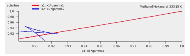
Thus there is a calculated miscibility gap. The properties of the two immiscible liquid phases are given in the table: the calculated miscibility gap is between approximately x1 = 0.275 and x1' = 0.811, with a calculated total vapor pressure of approximately 1.48 bar. Within the miscibility gap, the liquid mixture consists of 2
