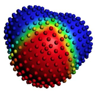
The small spheres represent the COSMO surface points that are used for the construction of the COSMO surface.
