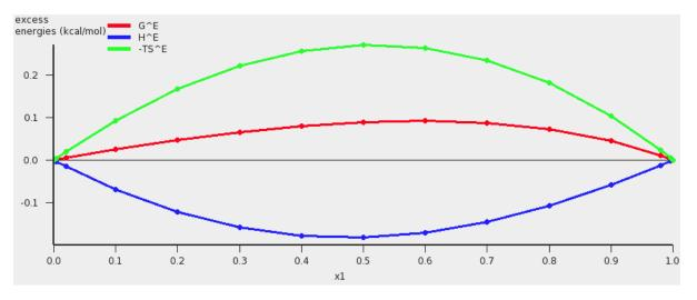
The red curve is the excess Gibbs free energy  $G^{E}$ , the blue curve is the excess enthalpy  $H^{E}$ , and the green curve is -T times the excess entropy  $S^{E}$ .
