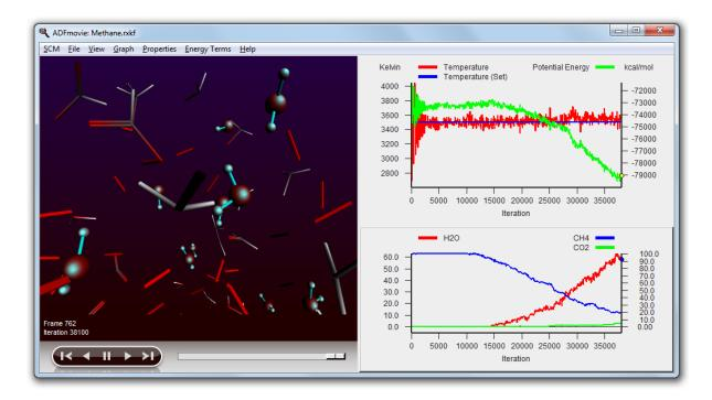
Wait until the calculation is ready Select the CO2 curve (click on it) Move it to the left axes: Graph  $\rightarrow$  Curve On Left Axes
