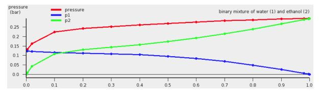
The red curve is the total vapor pressure, the blue curve is the partial water vapor pressure, and the green curve is the partial ethanol vapor pressure. One can also change the x and y axes, for example:
