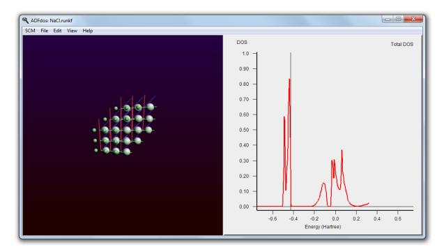
The Fermi energy is around -0.43, and there is clearly a gap. Just below it there is a valence band, and at -0.2 Hartree starts the conduction band.
