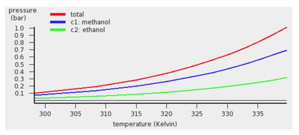
The red curve is the total vapor pressure, the blue curve the partial methanol vapor pressure, and the green curve is the partial ethanol vapor pressure. The table gives the numerical values.
