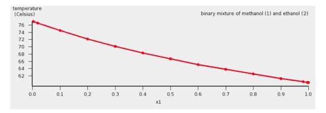
If one clicks in the graph window at the left or below the axes, a popup window will appear in which one can set details for the graph window. In the graph above the 'Units' for the 'Left Y Axes' were chosen to be 'Celsius'.
