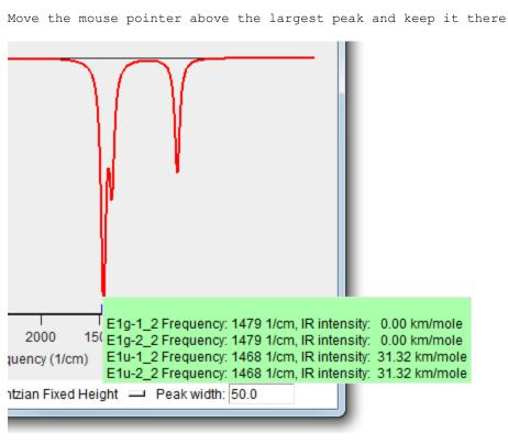
The list of normal modes contributing to the IR peak will show up. By clicking the mouse button at this point, the first of these modes will be showb by animating the ethane molecule on the left. Alternatively, pressing and holding the mouse button down, a list of these modes with their symmetry labels will show up:
