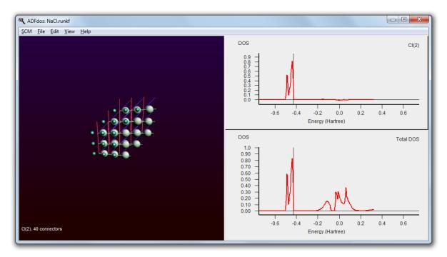
It is already immediately clear that the valence band comes from the Chlorine, and the conduction band from the Sodium.
