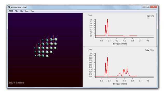
Right-click with the mouse on the selected Cl atom and check the 'P-DOS' check box in the pop up menu.
