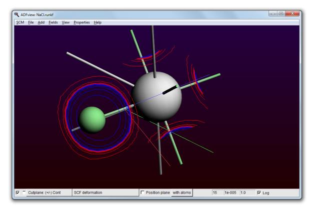
Indeed we see that charge is added (blue) near the CI and removed (red) from the Na atom. The trend is good, but what is the total amount of charge transferred?
