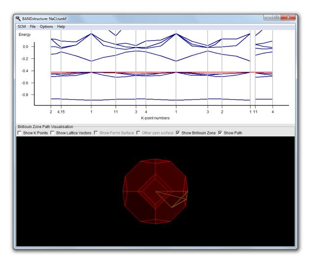
It consists of a plot and a picture of the Brillouin zone. In the plot the red line is the Fermi level. Below the Fermi level are four occupied bands. You can see this more clearly by vertical zooming:
