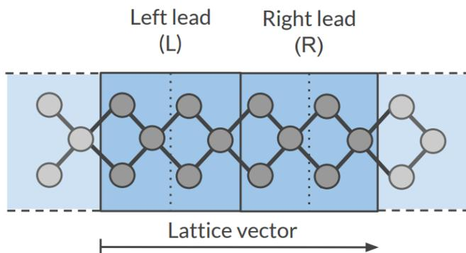
A tight binding (TB) representation is calculated for the overlap ( $S(R = 0)$  and  $S(R = a)$ ) and Fock matrix ( $H(R = 0)$  and  $H(R = a)$ ). This is not an approximation provided that the functions do not extend beyond the neighboring cells. You should choose a sufficiently large super cell for this to be true. For this reason we recommend setting the *SoftConfinement* (page 46) Quality to Basic, thus reducing the range of the functions.
