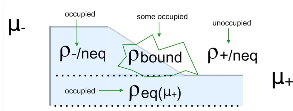
Fig. 7.2: Figure: The non-equilibrium density consists of three parts: the left and right parts ( $\rho_{-/neq}$  and  $\rho_{+/neq}$ ) and the bound states ( $\rho_{\text{bound}}$ ). We want to know the occupied part.
