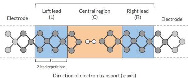
Our goal is to compute the **transmission function** T(E), which describes the rate at which electrons of energy E are transferred from the left electrode to the right electrode by propagating through the scattering region. From the transmission function we can calculate the electric current for given **Bias Voltage** V applied between the electrodes:
