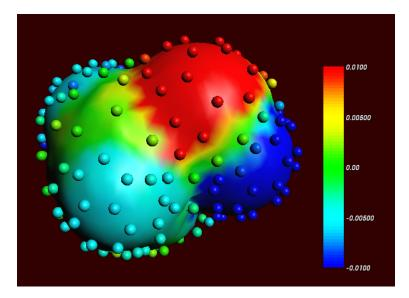
Cosmo charge density on the COSMO surface of methanol, Esurf surface (picture made with AMSview).
