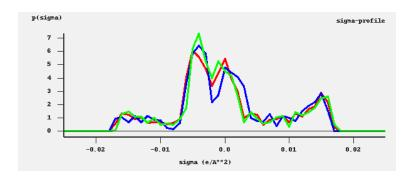
$\sigma$ -profiles of methanol (picture made with the CRS-GUI). In this picture the blue line is the  $\sigma$ -profile with the Esurf type of construction, the red line is that with the Delley type of construction with many surface points. For comparison, the green line is the  $\sigma$ -profile of methanol if a large QZ4P basis set is used, again with the Delley type of construction with many surface points.
