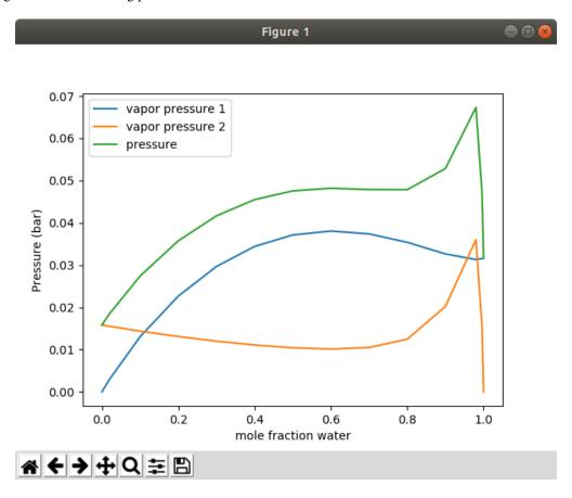
Fig. 10.4: A plot showing the total and partial vapor pressures for the water/2-Hexanone system.
