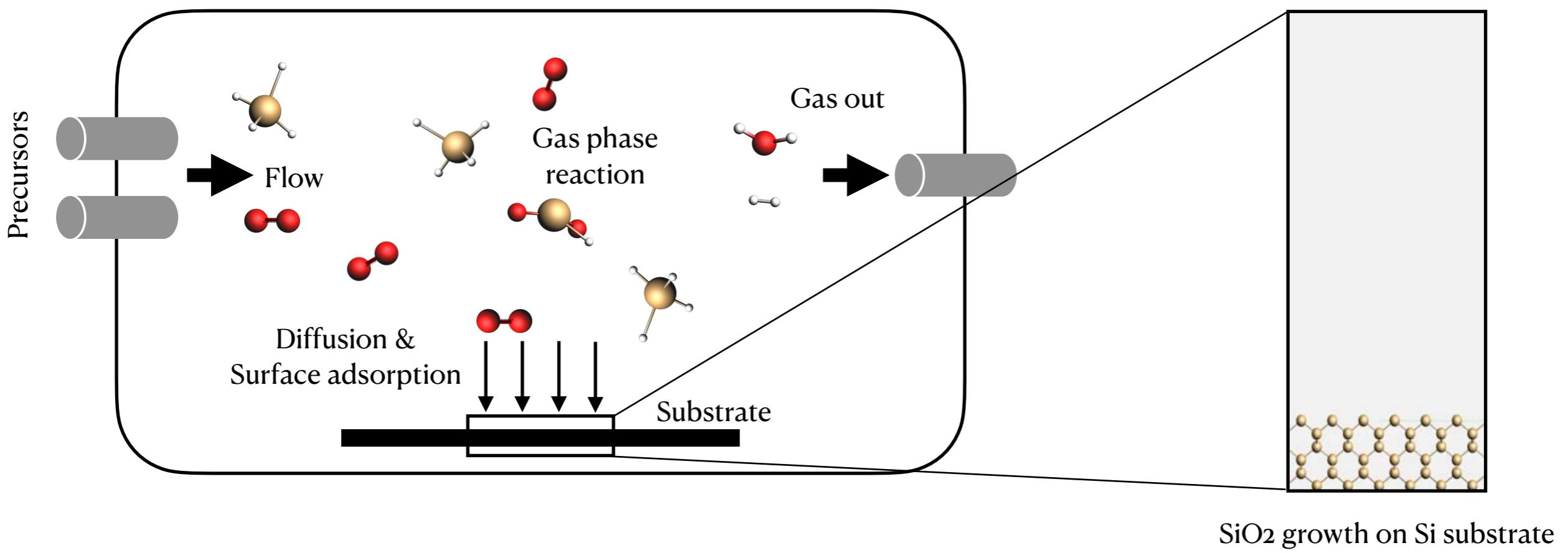
$\text{SiO}_2$  growth on  $\text{Si}$  substrate
