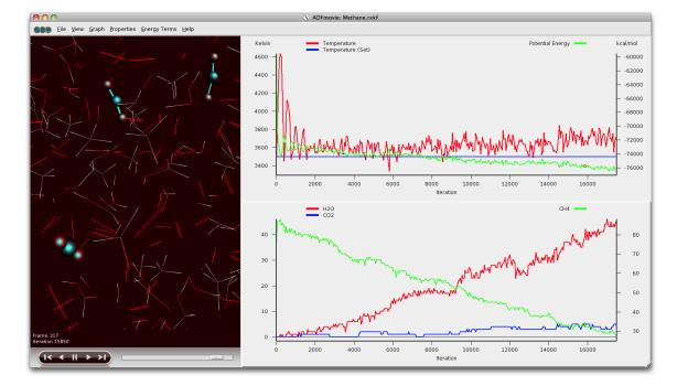
When you now go forward or backwards in time, it is easier to see how the reactions actually take place. Note that the atoms remain selected, even if they are no longer part of a CO2 molecule. In a similar way you can focus on H2O produced:
