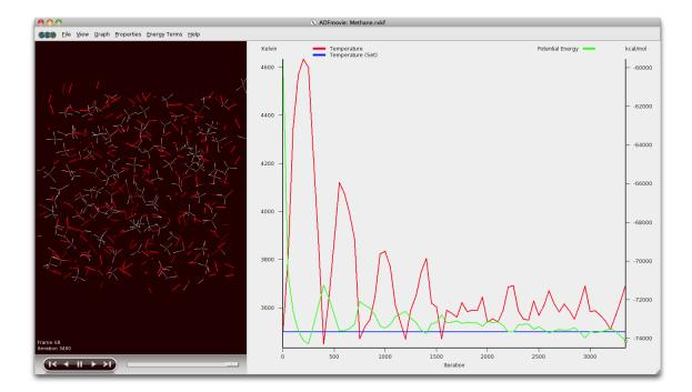
Note that the two temperatures (the actual temperature, and the set temperature) are both plotted on one axes. The other axes is used for the second property (in this case the potential energy).
