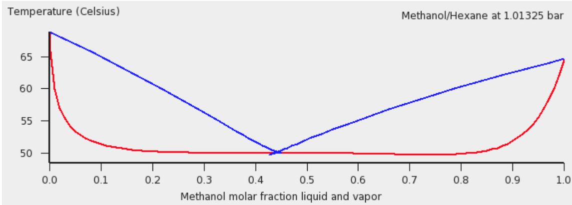
Experimental results for the Methanol-Hexane mixture were taken from Ref. [451]. These are compared with the calculated ones in the next graph. More experimental VLE data might also be found at Ref. [452].
