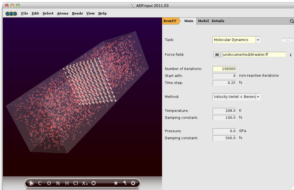
In the simulation we would like something to happen. So we will use a high temperature for water, but try to keep the aluminum cool. Also, we will start with a low temperature MD to relax the initial set-up. This can all be accomplished using a temperature regime, specifying different temperatures for different regions.
