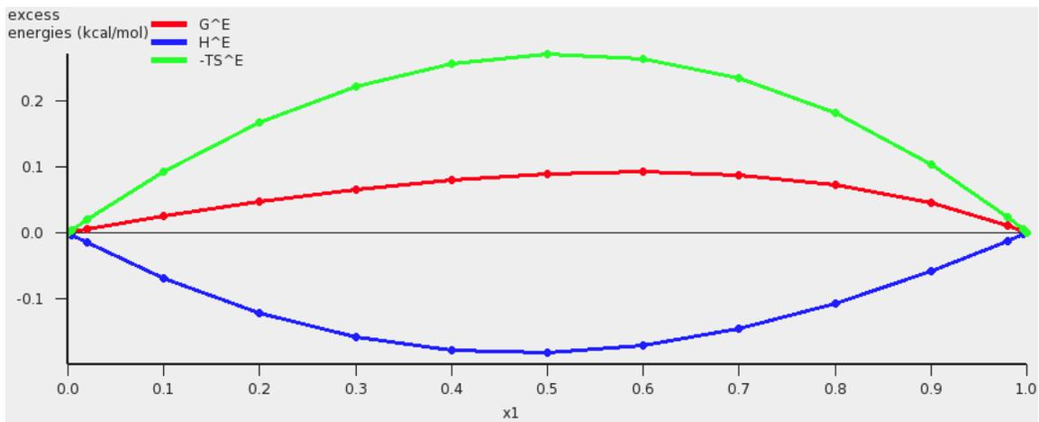
The red curve is the excess Gibbs free energy  $G^E$ , the blue curve is the excess enthalpy  $H^E$ , and the green curve is  $-T$  times the excess entropy  $S^E$ .
