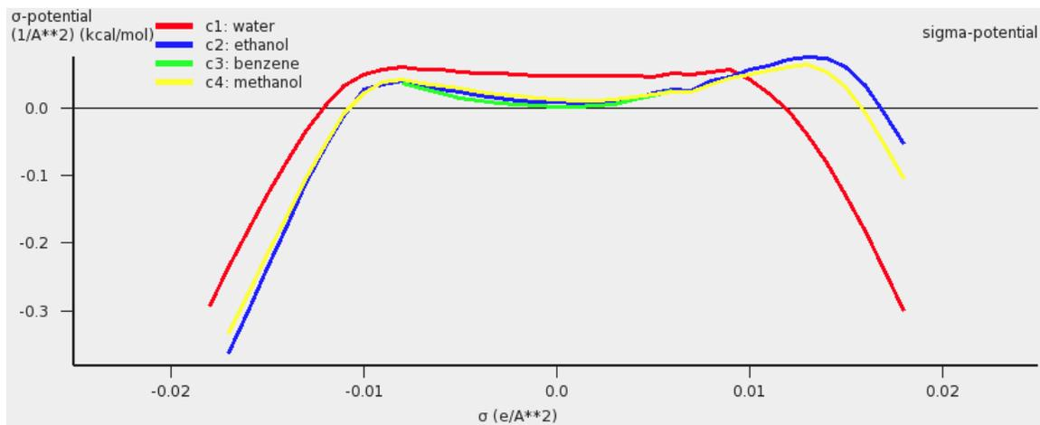
If the default settings are used, the red curve is the water  $\sigma$ -potential, the blue curve the methanol  $\sigma$ -potential, the green curve is the benzene  $\sigma$ -potential, and the yellow curve is the methanol  $\sigma$ -potential. In the details for the graph window the line widths for all curves were set to '3'.
