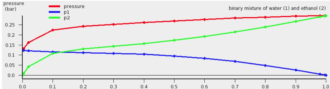
The red curve is the total vapor pressure, the blue curve is the partial water vapor pressure, and the green curve is the partial ethanol vapor pressure. One can also change the x and y axes, for example:
