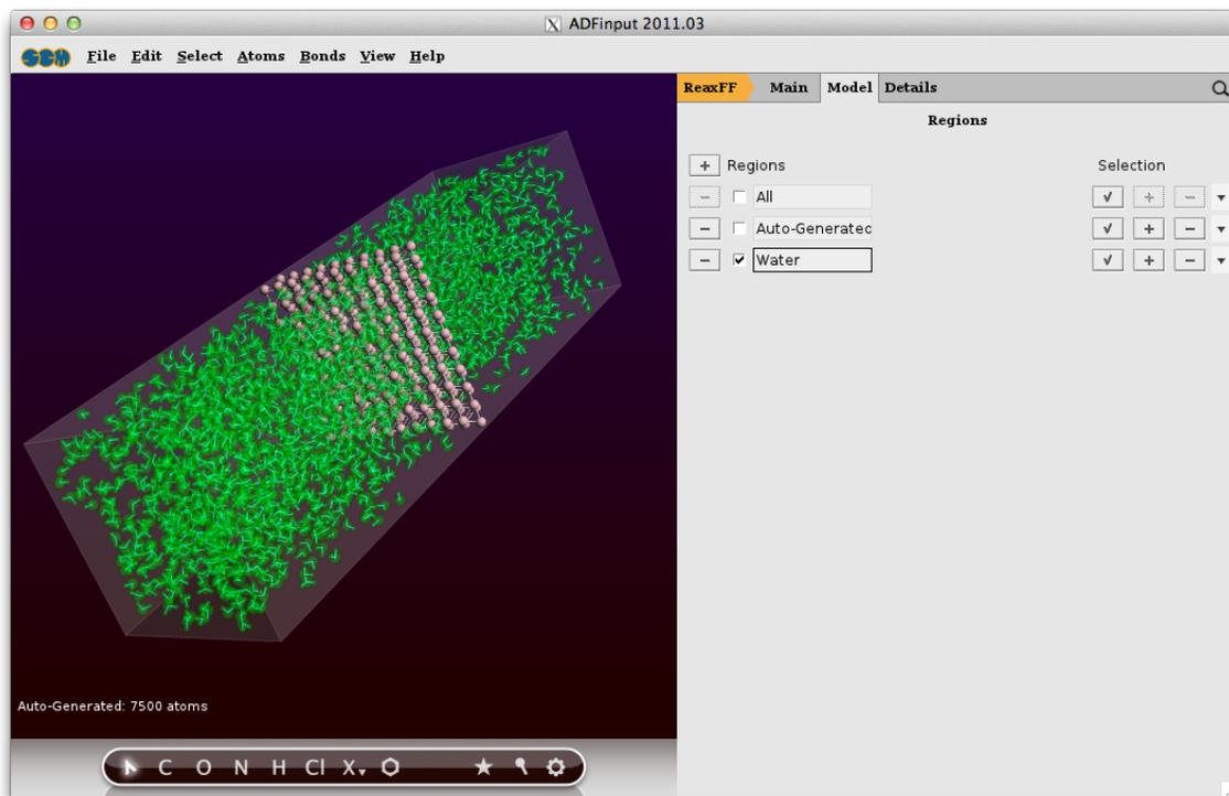
Now we have a region defined that contains all water molecules. Note that the selected atoms (in this case all water molecules) were automatically added to the new region. The + and - buttons add or remove the selected atoms to a region.
