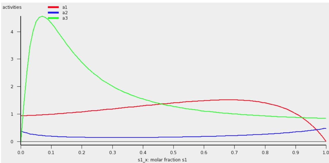
The activities of the pure compounds should be equal at the end point of a tie line  $a_1 = a_1'$ ,  $a_2 = a_2'$ , and  $a_3 = a_3'$ . If we look at the graph with close inspection this is approximately true for the molar fraction of solvent s1
