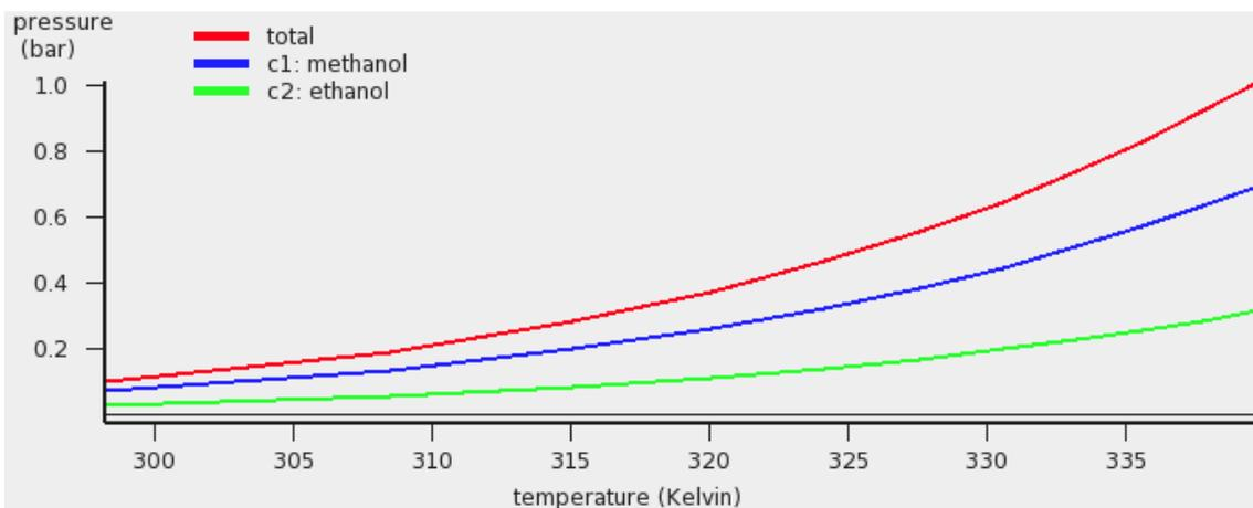
The red curve is the total vapor pressure, the blue curve the partial methanol vapor pressure, and the green curve is the partial ethanol vapor pressure. The table gives the numerical values.
