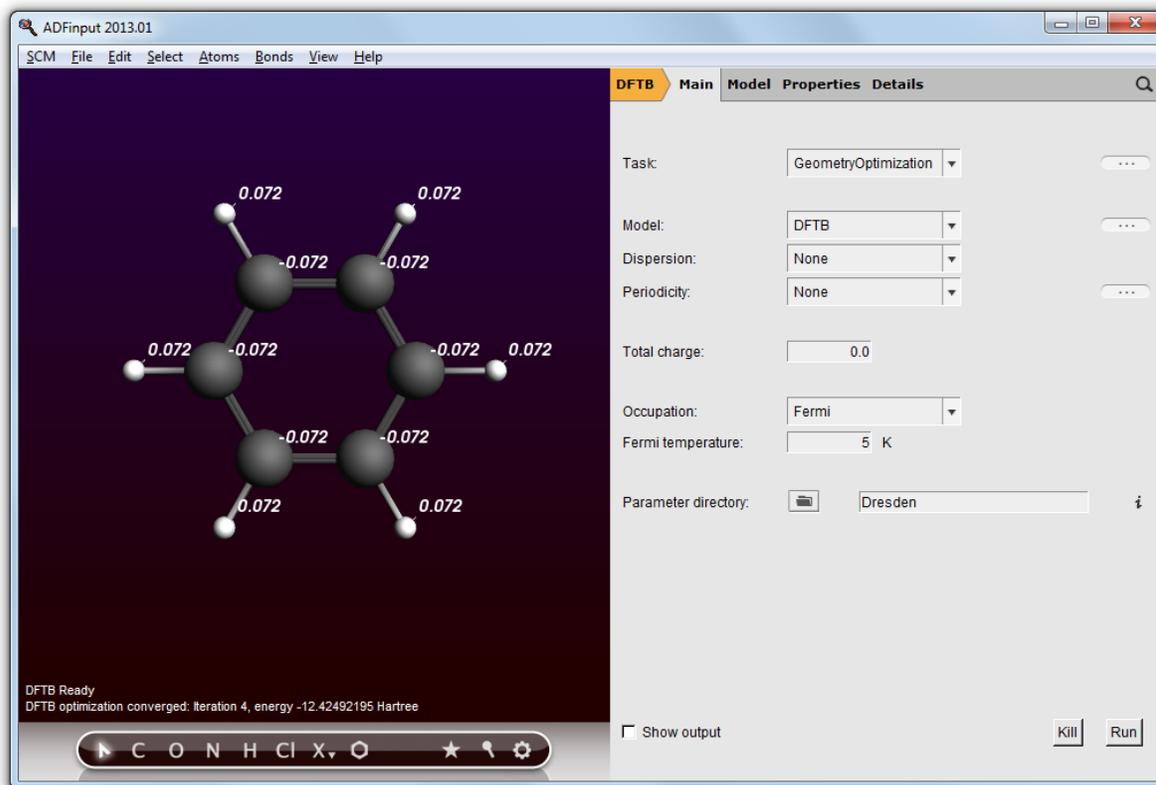
A Self Consistent Charge (SCC) evaluation allows atomic Mulliken charges to vary in an iterative procedure. This influences the DFTB Hamiltonian until self consistency of these charges is reached.
