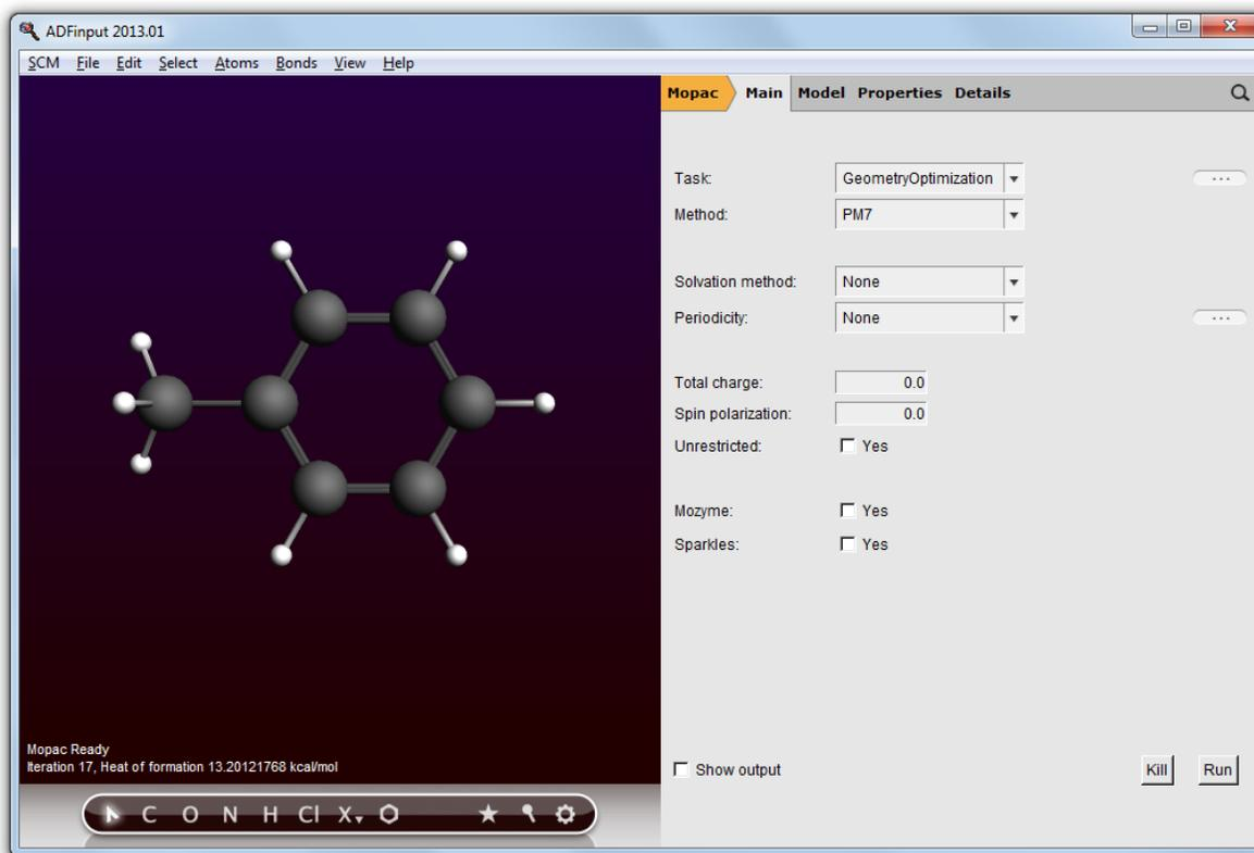
The geometry has been optimized, but as the starting geometry was very reasonable this did not lead to big changes. In the status area you can see that MOPAC used 17 iterations, and you can see the final heat of formation. And obviously the bonds reappeared. These bonds are actually based on the bond orders as calculated by MOPAC.
