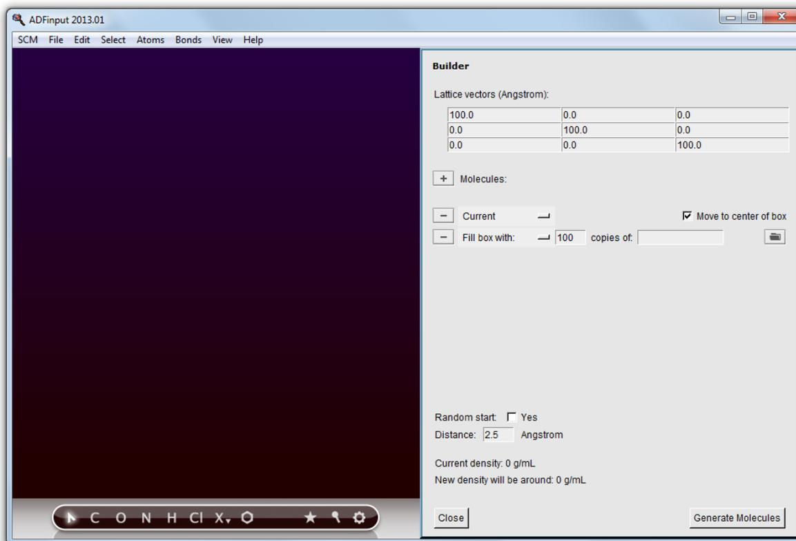
The Builder allows you to build your system, and set some things like the cell vectors that define the computation cell. ReaxFF always uses periodic boundary conditions. The default cell is a cube with sides of 100 Angstrom.
