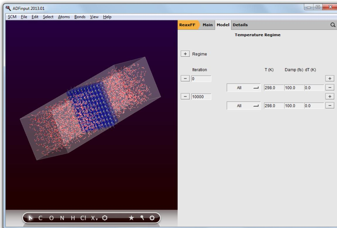
At iteration 0, we start with an MD simulation at T=0 K:
