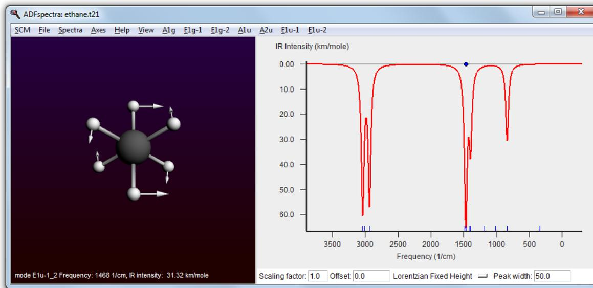
You can make the vectors larger or smaller using the same ctrl/cmd-L/K, or arrow up and down.
