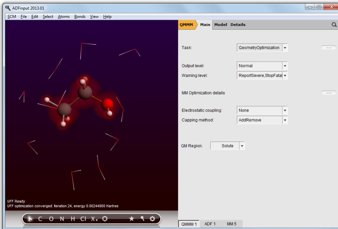
Now you will have three tabs: the main QMMM tab that allows you to set QMMM details, the 'ADF 1' tab that is the setup for the ADF calculation for the Solute subsystem, and the 'MM 5' tab that sets up the MM calculation for the full system.
