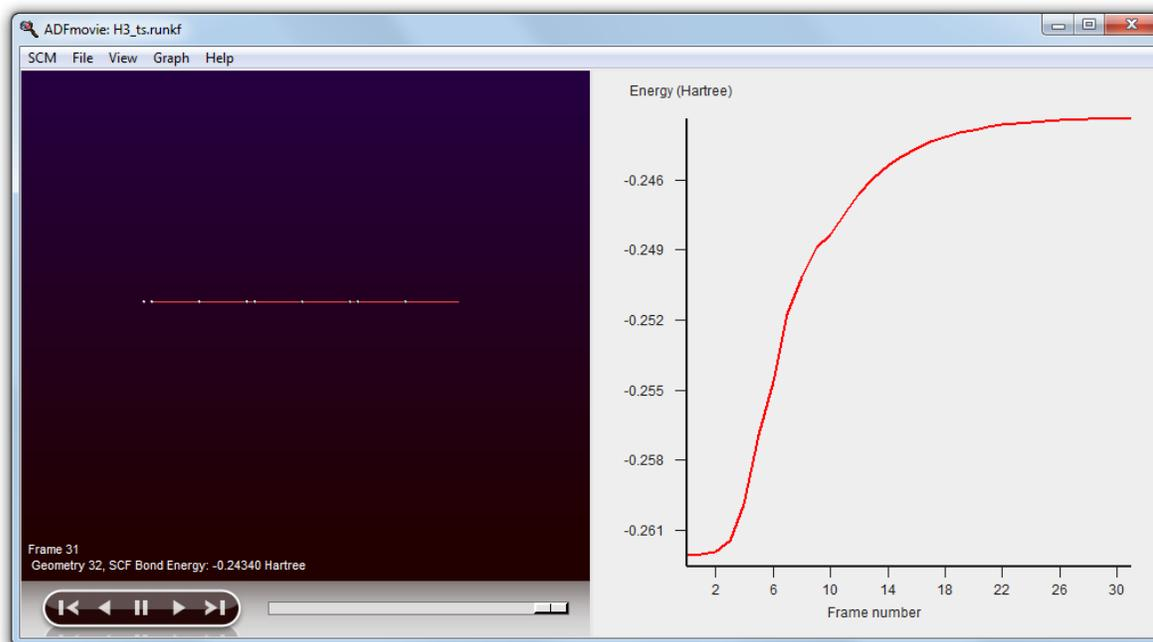
The third H atom ends up exactly in the middle of the (repeated) H1 and H2 atoms. Let us finally check that we are indeed in the transition state.
