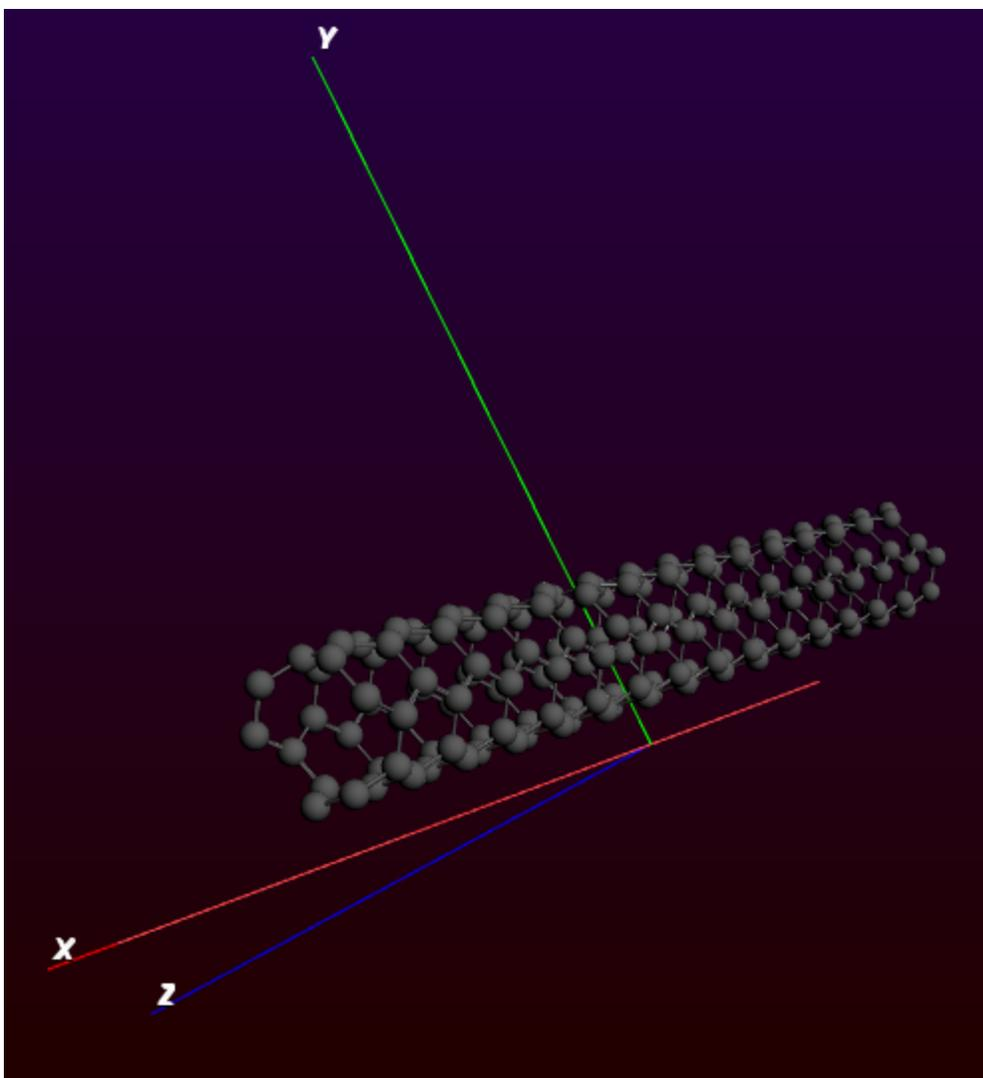
Switch to some non-periodic code (like ADF) if you wish to treat this piece of nanotube without infinite symmetry.
