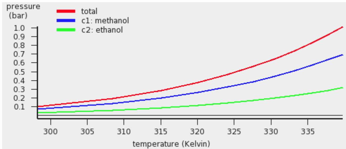
The red curve is the total vapor pressure, the blue curve the partial methanol vapor pressure, and the green curve is the partial ethanol vapor pressure. The table gives the numerical values.
