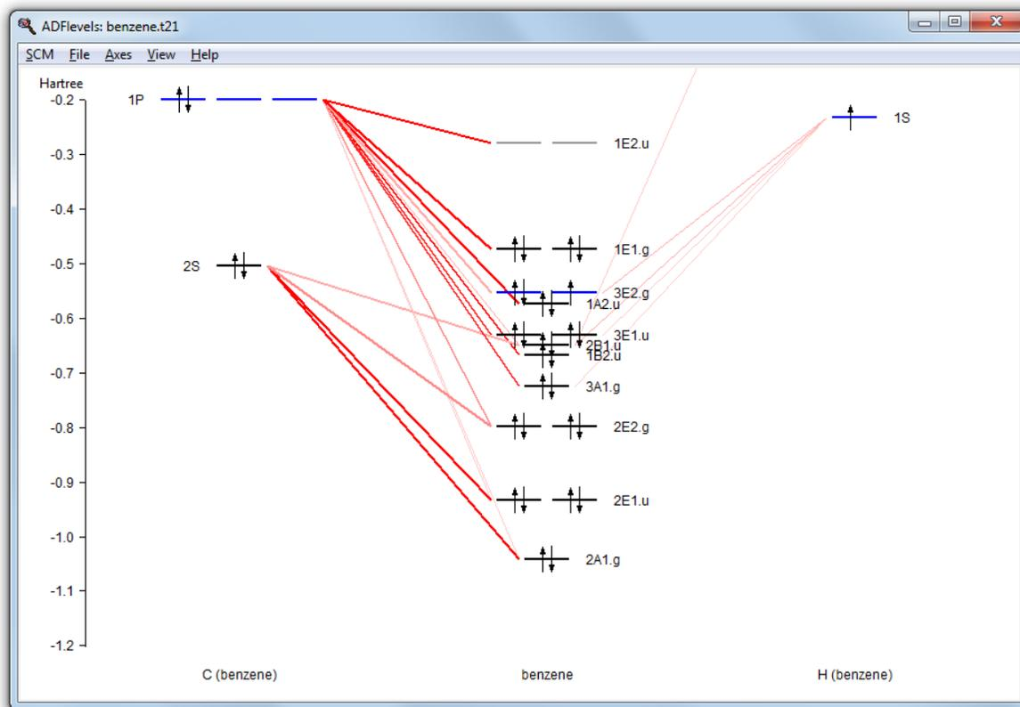
In the levels diagram you will observe that the HOMO (the 1E1.g) is completely filled, while the orbital below it has a hole. You can easily see this by the color. Note that we have performed a restricted calculation, so in effect the hole is averaged over the E orbitals.
