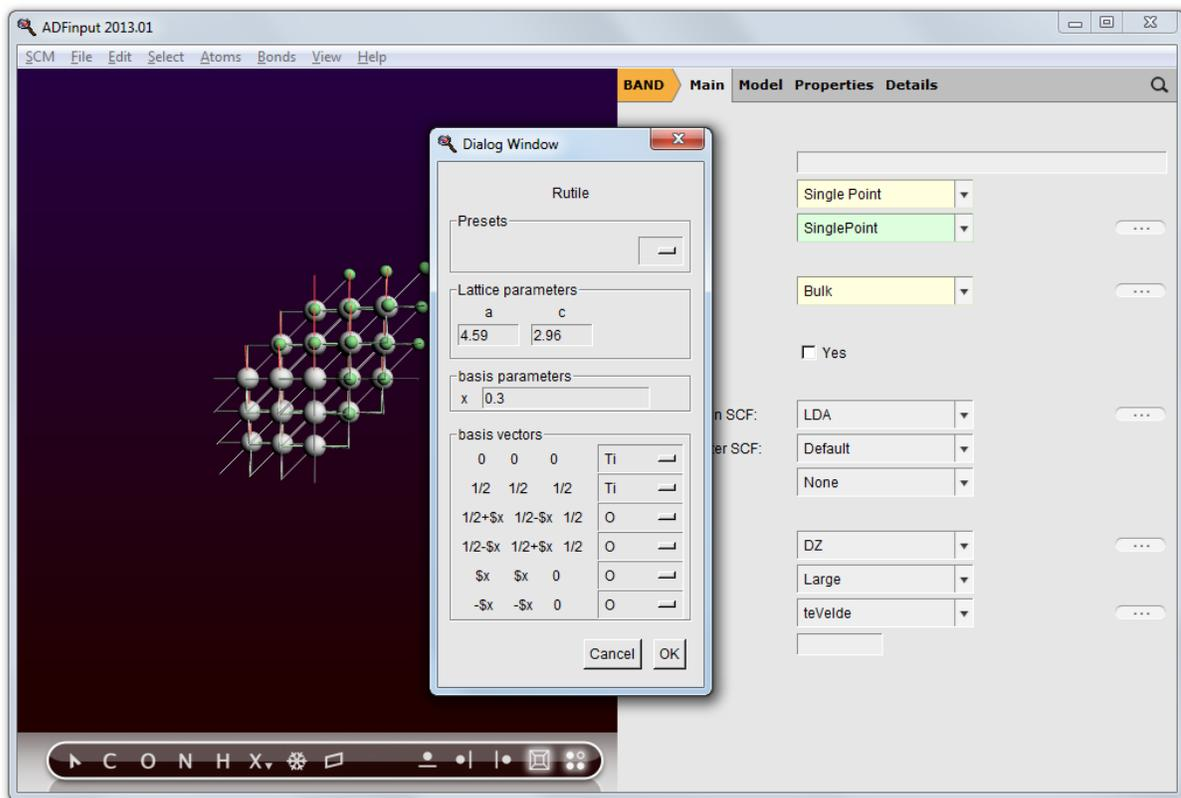
As you can see, it has two lattice parameters that need to be specified. But now also the positions of the oxygens have a parameter "x"
