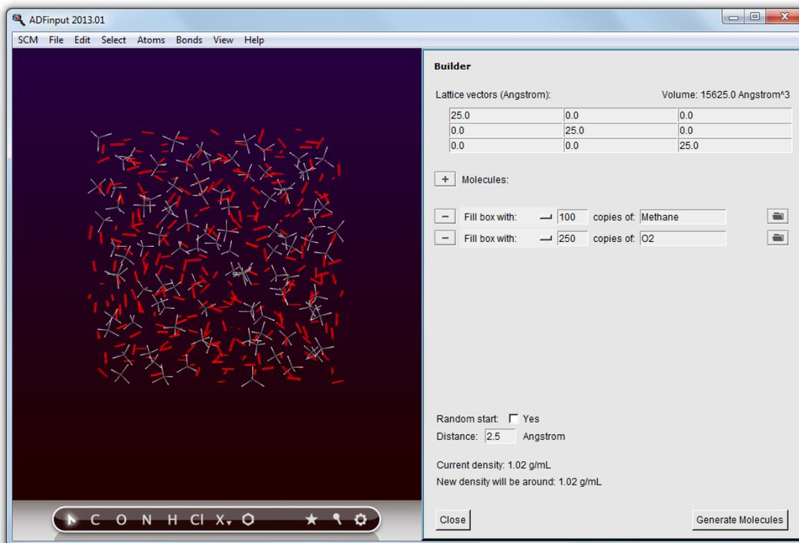
The molecules are generated at random positions and orientations, with constraint that all atoms (between different molecules) are at least the specified distance (2.5 Angstrom) apart.
