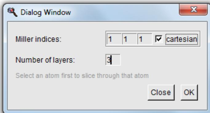
The "Cartesian" option is needed because the Miller indices are usually (with cubic lattices) thought in the conventional unit cell rather than the primitive (minimal) unit cell.
