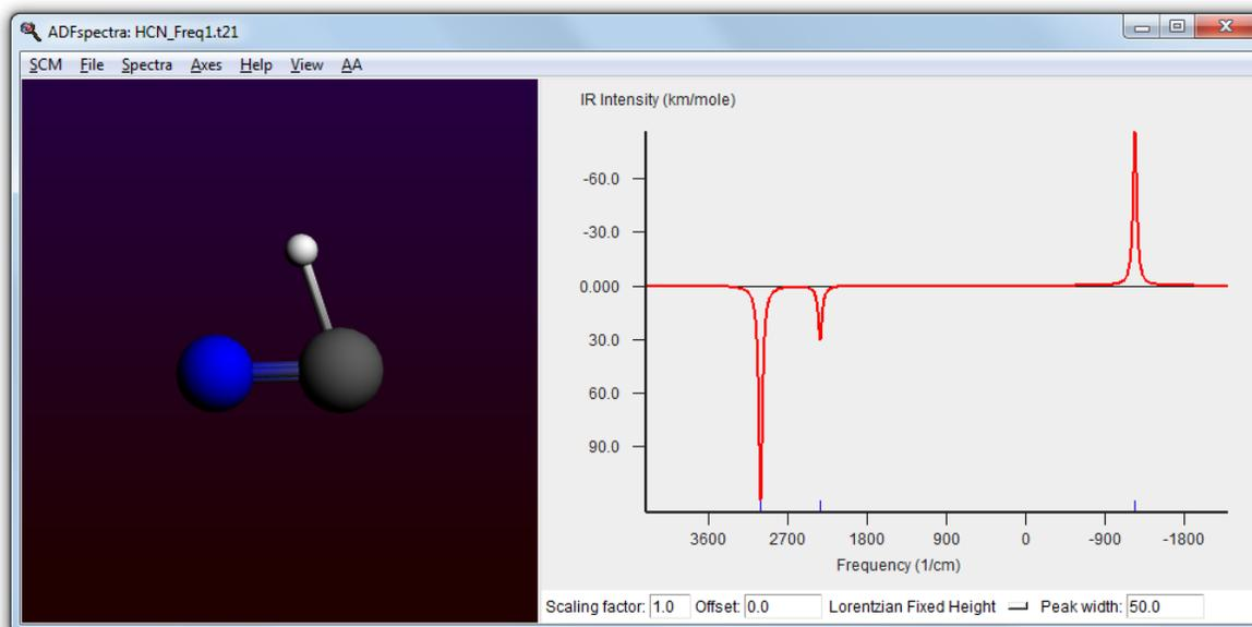
If everything was done correctly, you should see a spectrum with three peaks: two in the range of 2000 - 3000 1/cm and one peak in the range of negative or very low positive values. A negative frequency value actually means that it is an imaginary frequency.
