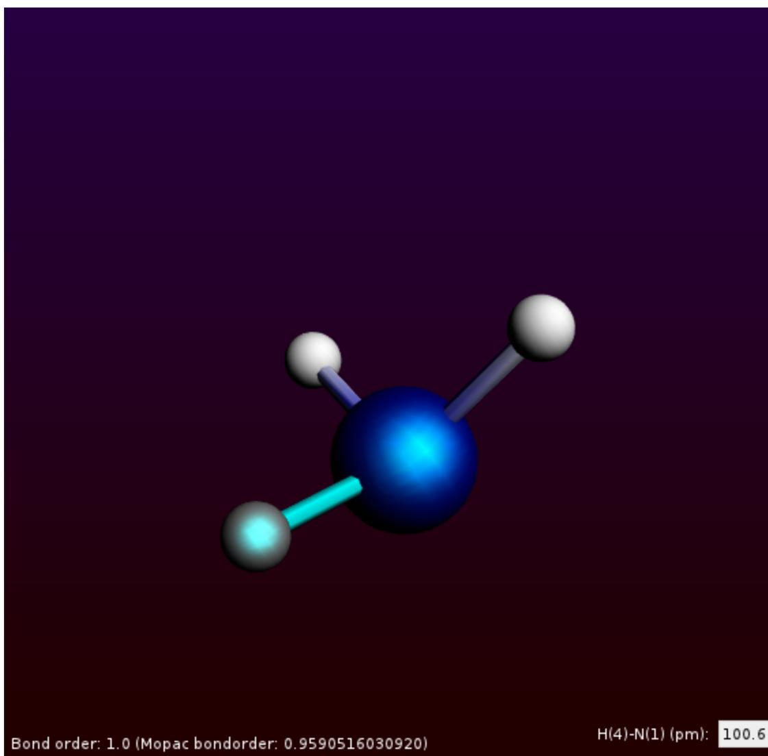
Mopac will produce a good-looking pyramidal ammonia molecule, with the N-H bond length of about 1.0 Angstrom.
