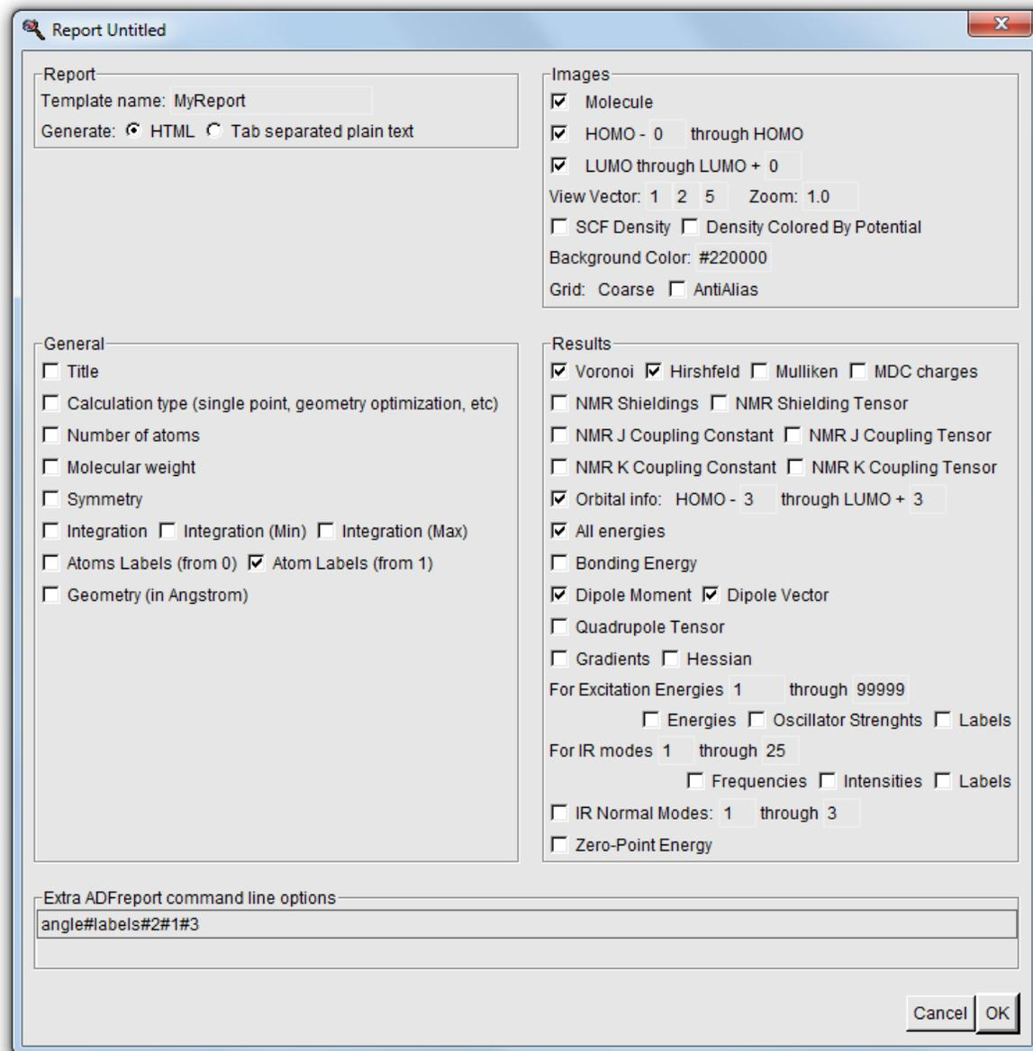
The extra command line options used instruct ADFreport to report the angle between atoms 2, 1 and 3, and include the atom labels for this angle on output. In a similar way more angles could be requested, or distances, or many other properties. For a description of all options please check the adfreport documentation.
