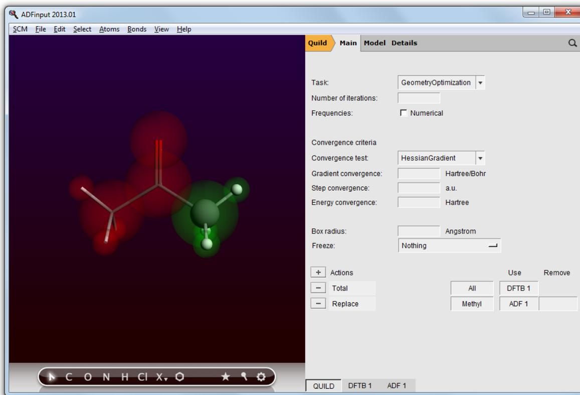
The first action ('Total') defines what to do with the full molecule. It normally will apply to the entire molecule, and thus the 'All' region is preselected. In the 'Use' field you have specified how to treat the whole molecule: with DFTB.
