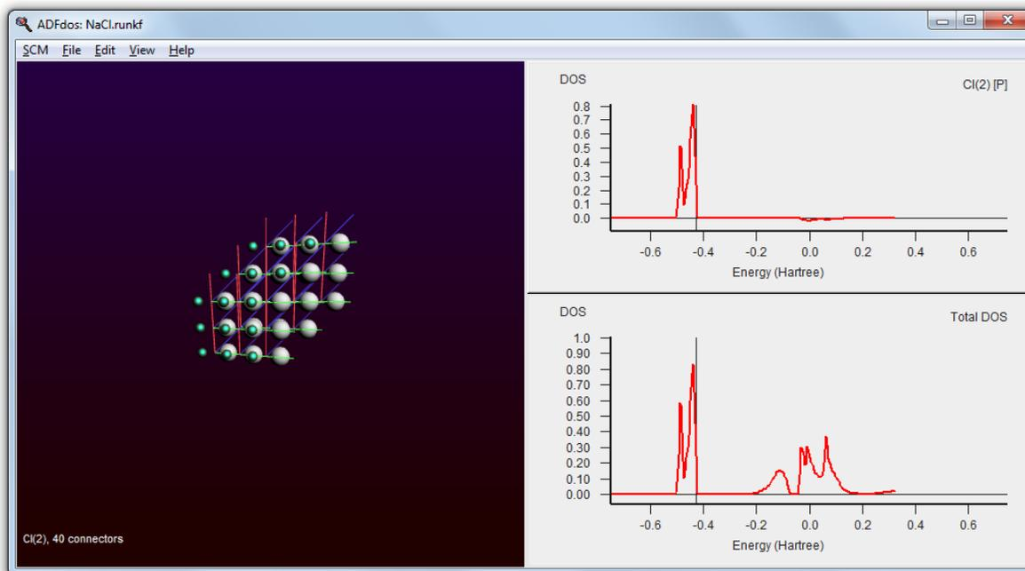
This shows that the valence band is clearly made of Chlorine p-orbitals.
