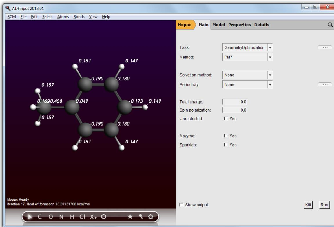
To see the MOPAC output, check the 'Show output' check box. And there is another way to run MOPAC interactively: use the pre-optimizer button (the cog wheel).
