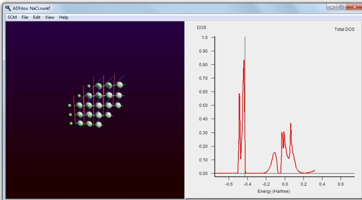
The Fermi energy is around -0.43, and there is clearly a gap. Just below it there is a valence band, and at -0.2 Hartree starts the conduction band.
