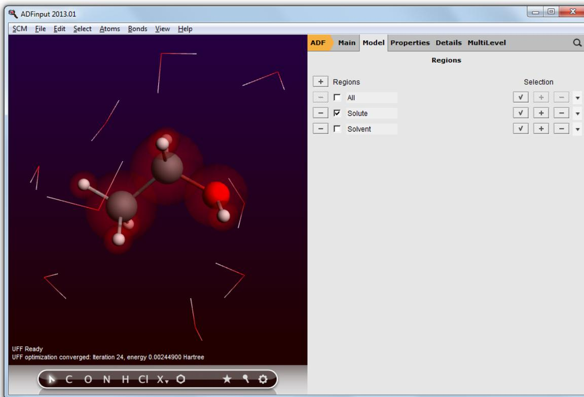
As you can see, ADFinput has generated 10 water molecules around your ethanol molecule. It also has created two regions: a Solute region containing the ethanol molecule, and a Solvent region containing the water molecules. The visualization option for the Solvent region is such that the water molecules will only be shown using a Wire-frame representation.
