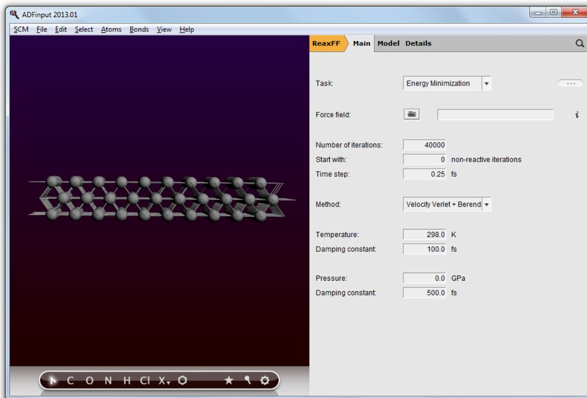
Now we have a real slab of aluminum, three layers thick. Note that the Generate Super Cell command adjusted the lattice vectors to match the new unit cell.
