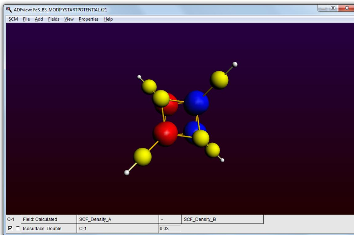
Note that you now have two visualization lines: one is a calculated field that actually calculates the difference between the alpha and beta spin density. The other is a double isosurface that visualized the calculated field. You can use these calculated fields for many purposes. For example, by changing the '-' into a '+' you are visualizing the total density instead of the spin difference density.
