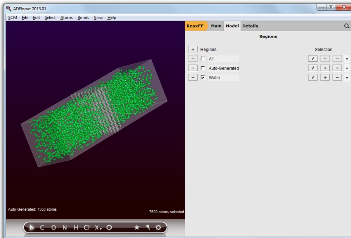
Now we have a region defined that contains all water molecules. Note that the selected atoms (in this case all water molecules) were automatically added to the new region. The + and - buttons add or remove the selected atoms to a region.
