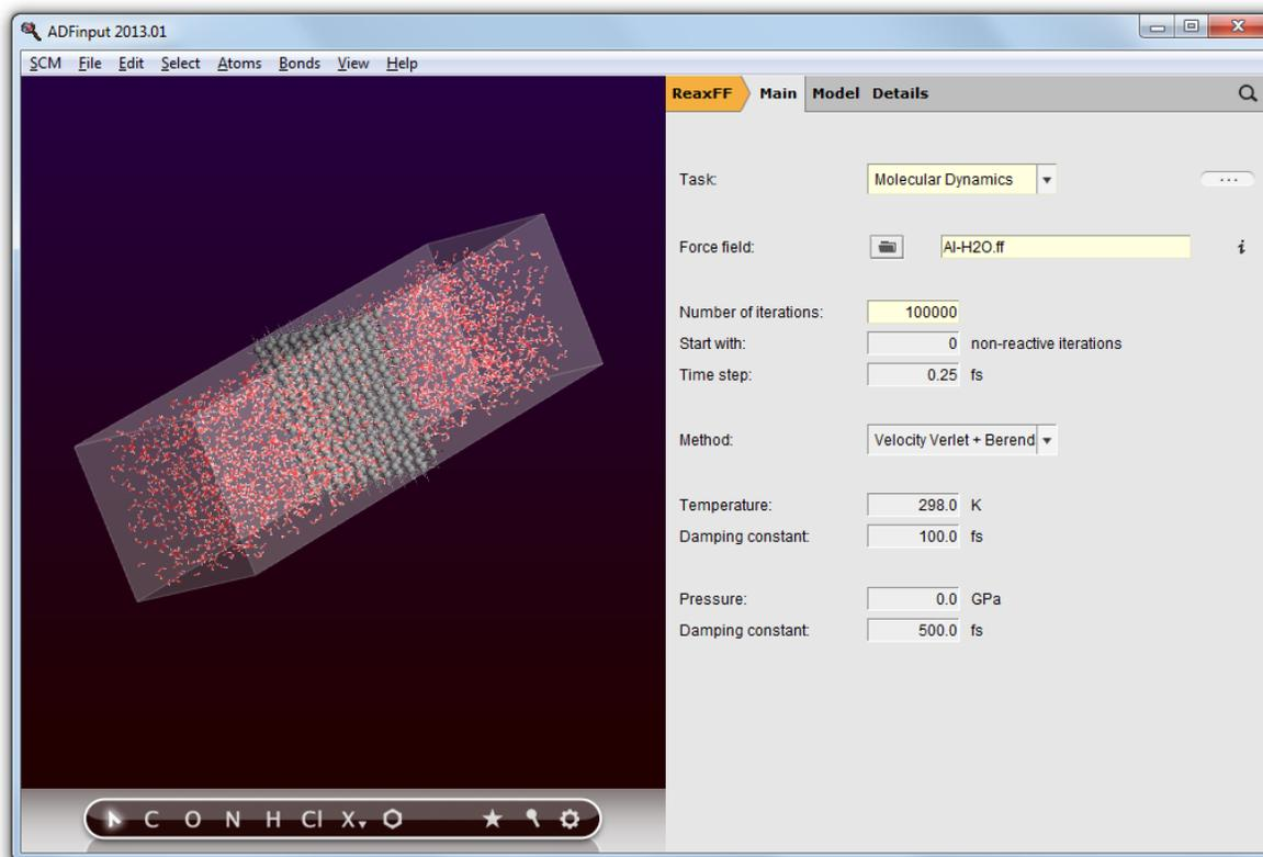
In the simulation we would like something to happen. So we will use a high temperature for water, but try to keep the aluminum cool. Also, we will start with a low temperature MD to relax the initial set-up. This can all be accomplished using a temperature regime, specifying different temperatures for different regions.
