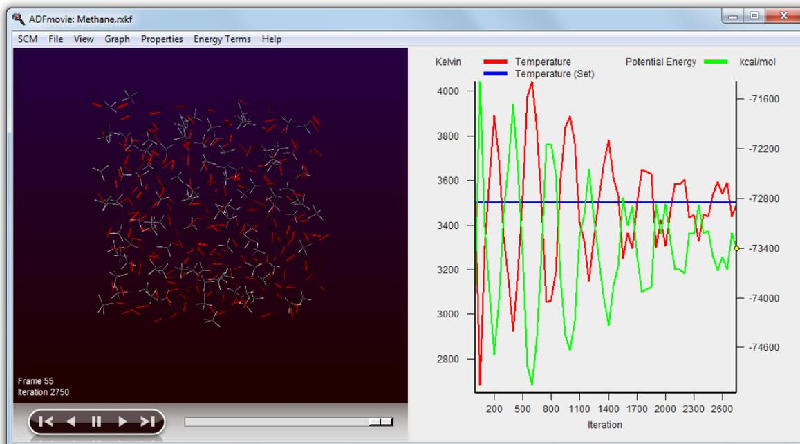
Note that the two temperatures (the actual temperature, and the set temperature) are both plotted on one axes. The other axes is used for the second property (in this case the potential energy).
