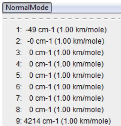
We have found a geometry with vanishing gradients with one weak negative vibrational mode. We have succeeded in finding a transition state.
