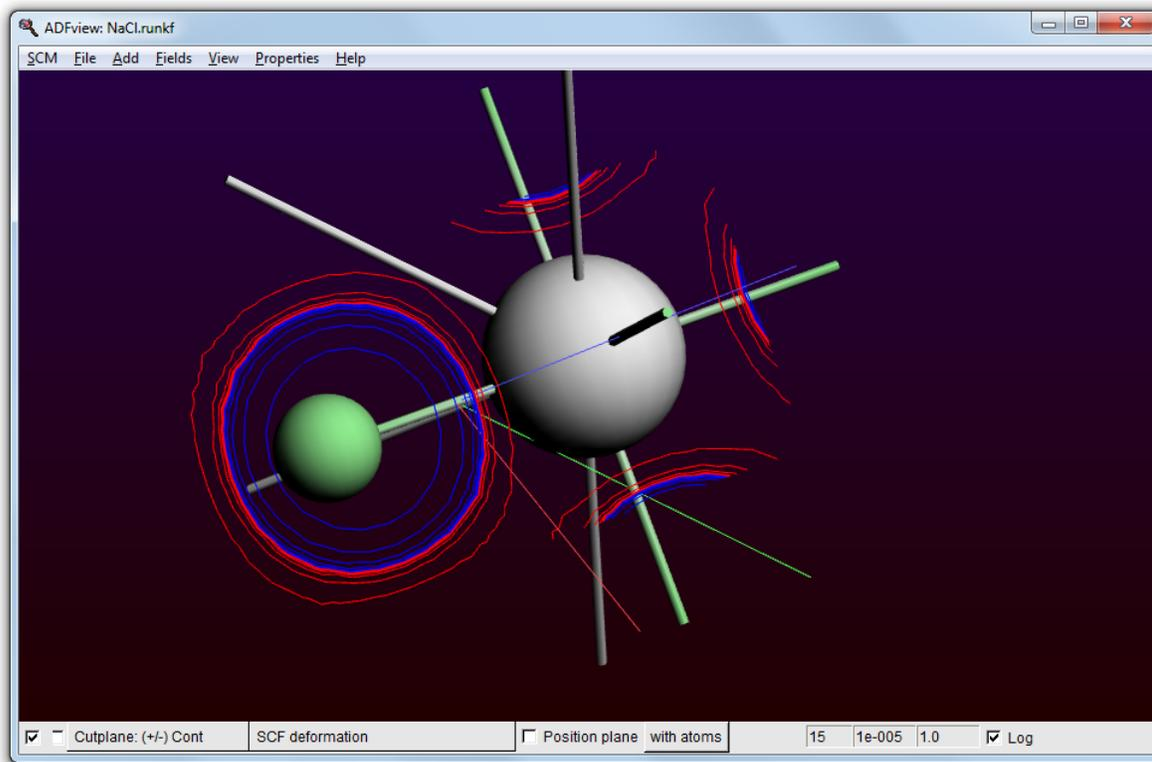
Indeed we see that charge is added (blue) near the Cl and removed (red) from the Na atom. The trend is good, but what is the total amount of charge transferred?
