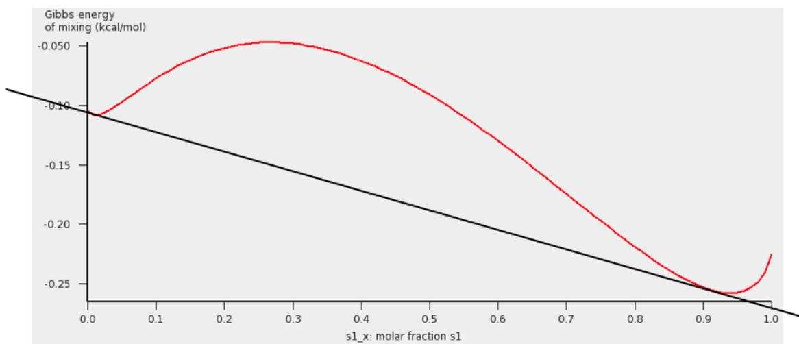
The black line was added to show the miscibility gap more clearly. Indeed at 67.9 °C for molar fractions between  $s1_x = 0.007$  and  $s1_x' = 0.91$ , the Gibbs free energy of mixing will be lower if the liquid has 2 phases.
