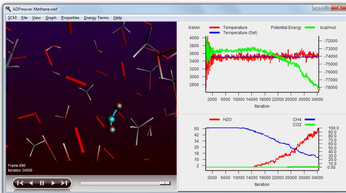
When you now go forward or backwards in time, it is easier to see how the reactions actually take place. Note that the atoms remain selected, even if they are no longer part of a CO2 molecule. In a similar way you can focus on H2O produced:
