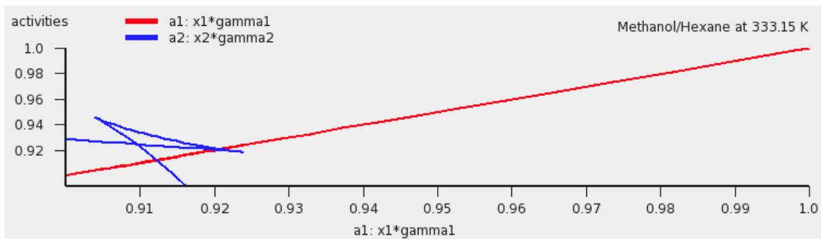
Thus there is a calculated miscibility gap. The properties of the two immiscible liquid phases are given in the table: the calculated miscibility gap is between approximately  $x_1 = 0.275$  and  $x_1' = 0.811$ , with a calculated total vapor pressure of approximately 1.48 bar. Within the miscibility gap, the liquid mixture consists of 2
