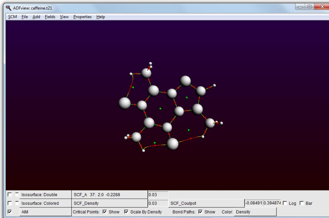
The critical points and bond paths are shown (the molecule balls and sticks representation is hidden). The different types of critical points (atom CP, bond CP, ring CP and cage CP) are indicated by different colors. The atom CPs are scaled by density by default, which makes them look like atoms. The bond paths are colored by density, by default.
