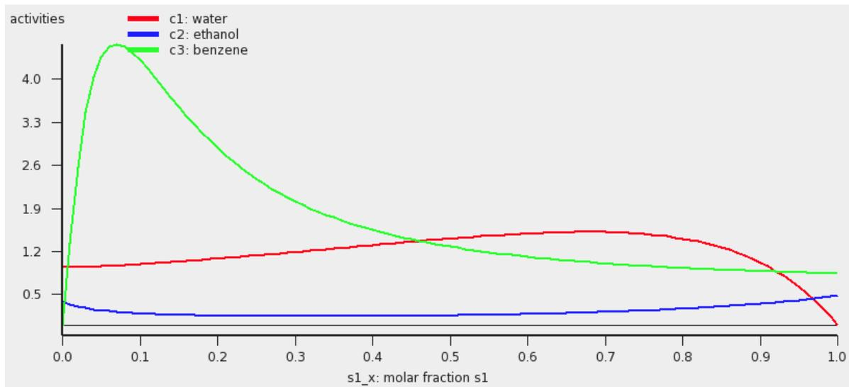
The activities of the pure compounds should be equal at the end point of a tie line  $a_1 = a_1', a_2 = a_2'$ , and  $a_3 = a_3'$ . If we look at the graph with close inspection this is approximately true for the molar fraction of solvent s1 with (approximately)  $s1_x = 0.007$  and  $s1_x' = 0.91$ . At a molar fraction of 0.91 of solvent s1 the calculated temperature is approximately 67.9 °C.
