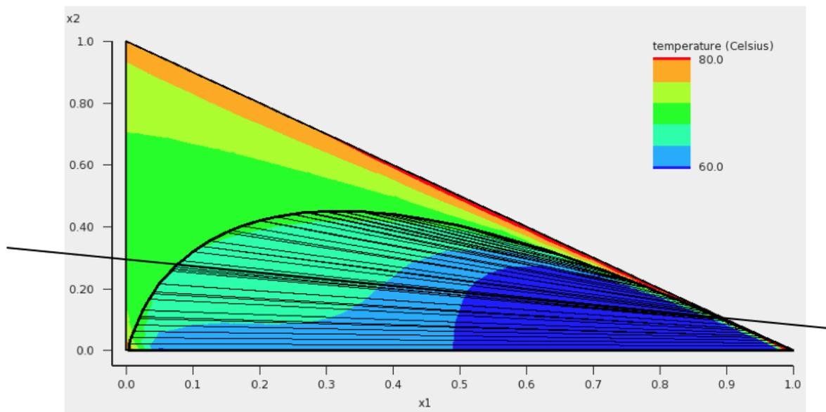
The compositions of solvents s1 and s2 are chosen where the black line in the picture above crosses the boundary of possible compositions. This means that solvent s1 and solvent s2 are mixtures of 2 compounds. Again experimental boiling points are used in the calculation.
