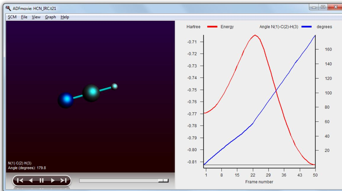
From this movie you can see the IRC path, and the energies at the most interesting points. As we have calculated the forward and backward path in one run, the order of the forward path needs to be reversed to get a proper energy graph.
