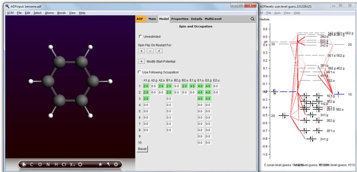
In the Spin and Occupation panel you see which orbitals are available (by symmetry, and spin if the current set up is unrestricted). The numbers are the occupations. Next to the ADFinput window ADFLevels will also have opened, and is showing a level diagram of your current molecule. This helps you to select the proper occupation.
