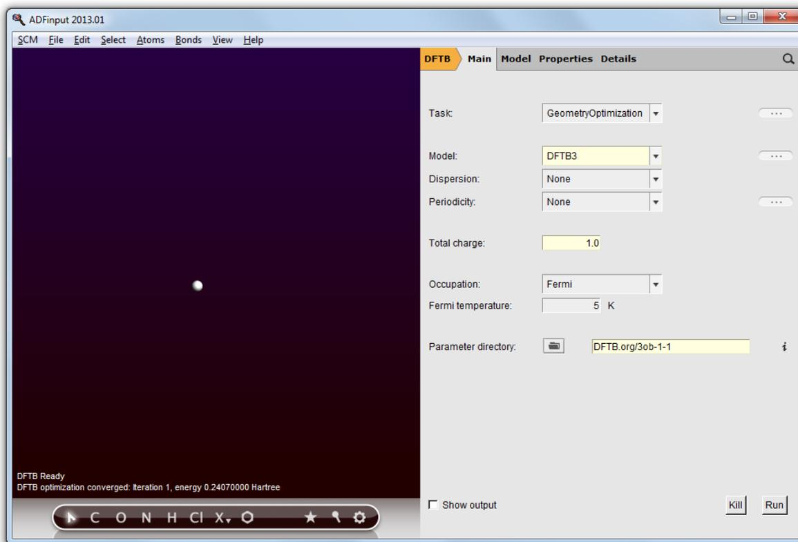
Finally, annotate the value for  $E(\text{H}^+) = 0.236417$  Hartree. The proton affinity is computed as  $\text{PA} = E(\text{Ac}^-) + E(\text{H}^+) - E(\text{HAc})$ , resulting in a final Proton Affinity of 0.566798 Hartree, or 355.67 kcal/mol.
