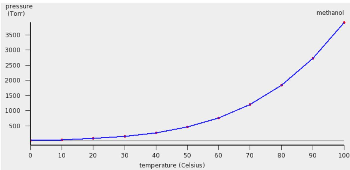
In this case COSMO-RS predicts a vapor pressure of about 0.61 bar (around 455 Torr) at 323.15 K (50.0 °C) for the pure liquid methanol.
