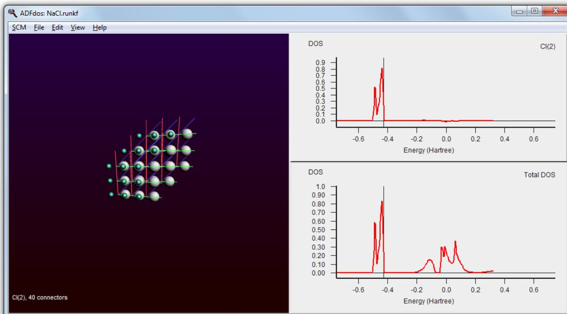
It is already immediately clear that the valence band comes from the Chlorine, and the conduction band from the Sodium.
