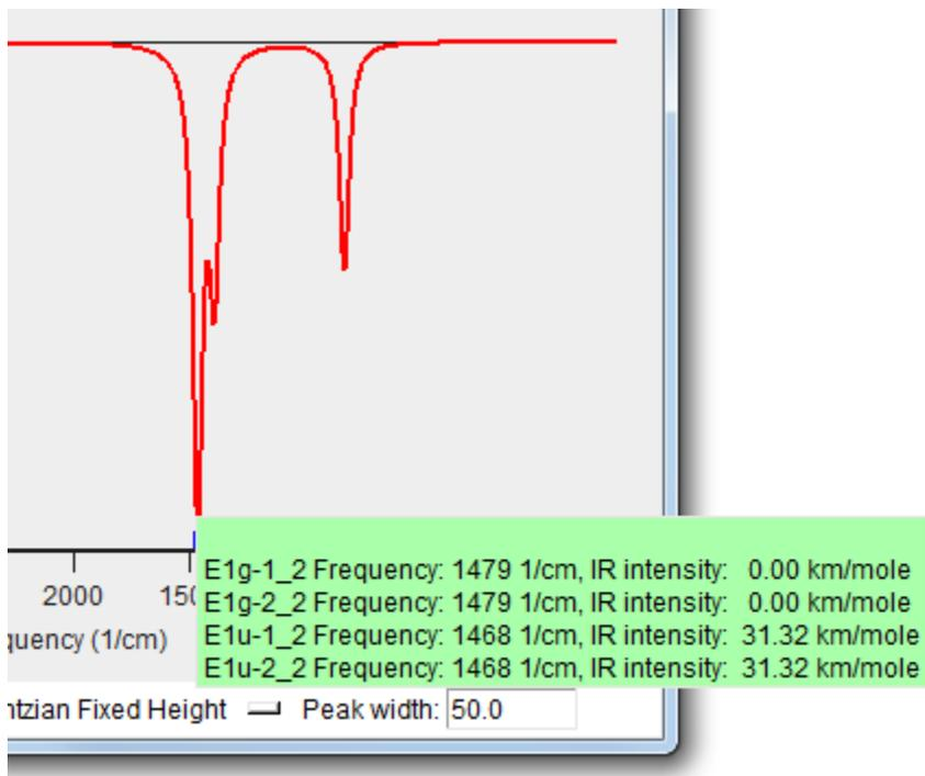
The list of normal modes contributing to the IR peak will show up. By clicking the mouse button at this point, the first of these modes will be shown by animating the ethane molecule on the left. Alternatively, pressing and holding the mouse button down, a list of these modes with their symmetry labels will show up:
