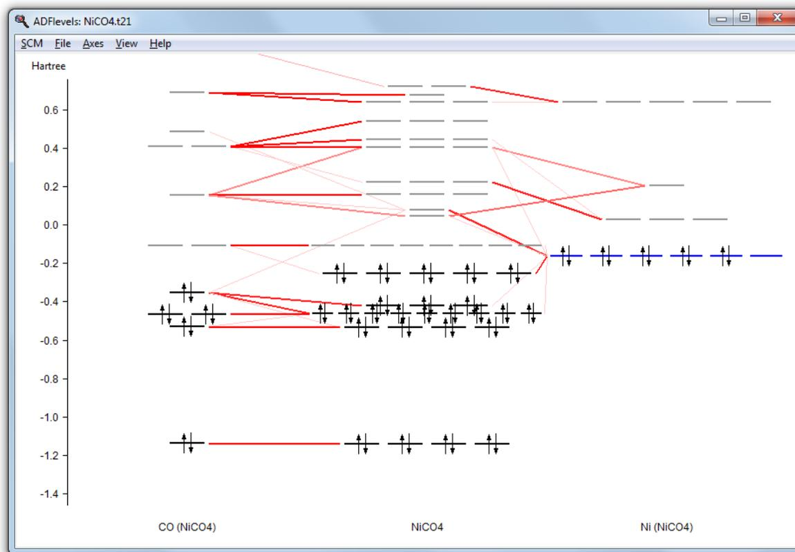
In the center you see the levels of the whole molecule, on the sides you see the CO fragment and the Ni-atom fragment. The interaction lines tell you which molecular orbitals come from which fragment orbitals.
