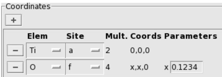
As you can see in the "Coords" column and the "Parameters" column, this site has an undetermined parameter "x". (It represents a symmetry line for this space group.) In the book you can find that for TiO<sub>2</sub> "x=0.3".
