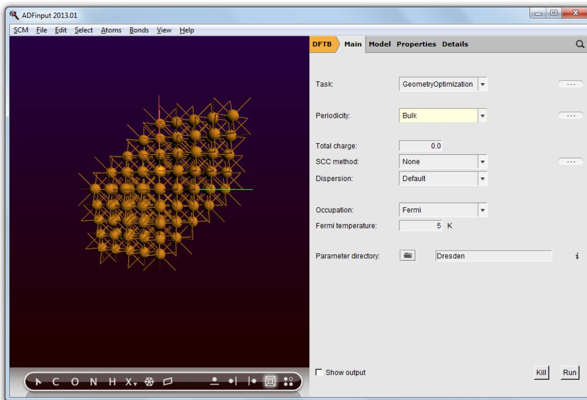
Now we have a block of Cu, with explicit Cu atoms (that is using a super cell). Next we will center this block, and select a sphere of atoms around the origin.
