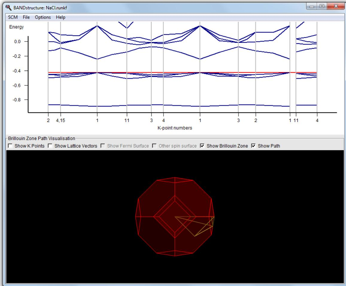
It consists of a plot and a picture of the Brillouin zone. In the plot the red line is the Fermi level. Below the Fermi level are four occupied bands. You can see this more clearly by vertical zooming:
