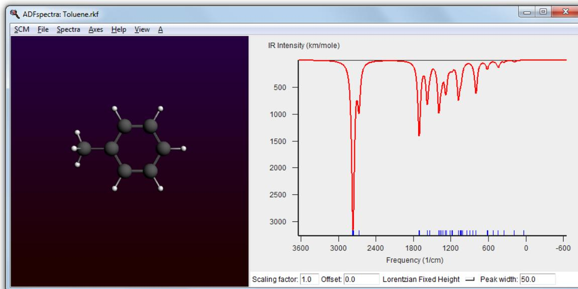
Right-click on the peak around 2762  $\text{cm}^{-1}$ , and select mode A\_37 (with the maximum intensity)
