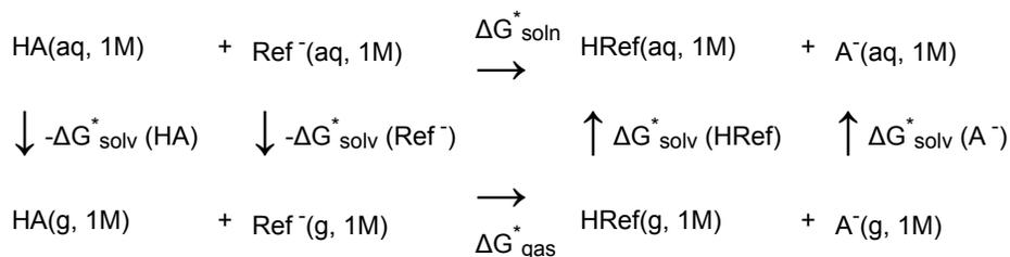
The \* denotes a standard state of 1M (1 mol/L). The free energy of solvation is then calculated as
