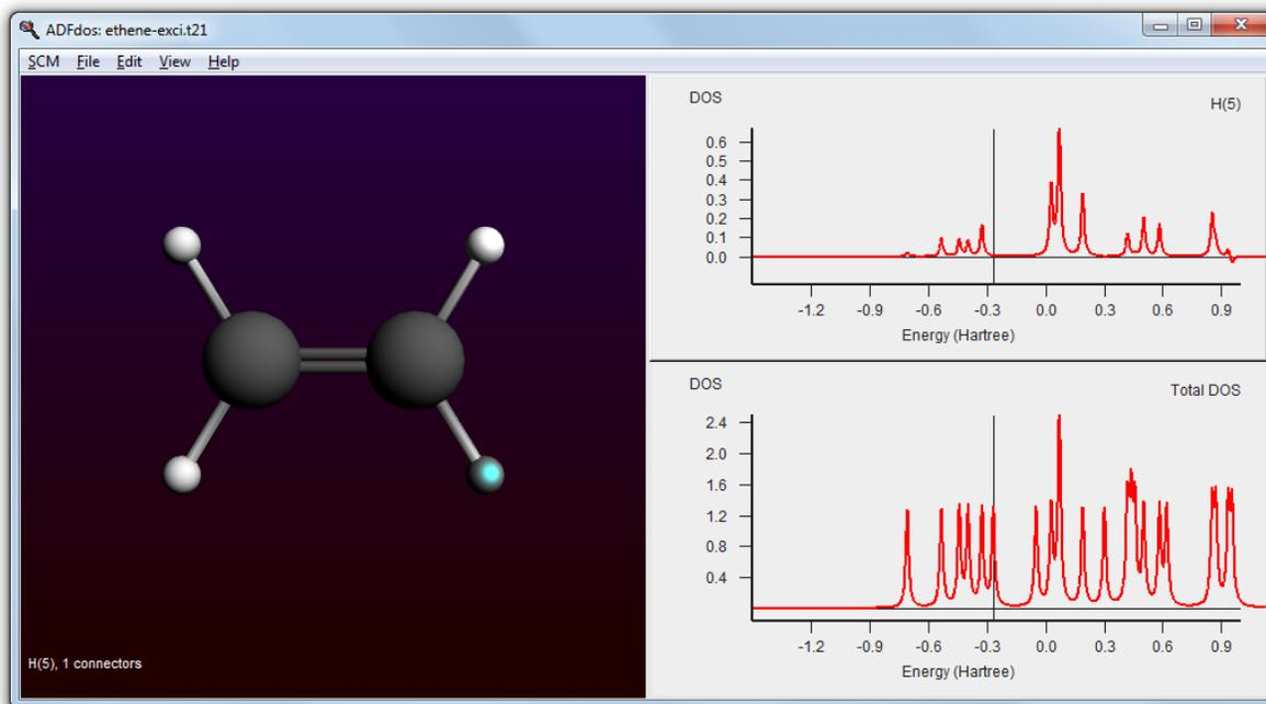
In these plots you can see that the partial DOS for the hydrogen atoms have no contribution to the HOMO. By right clicking on an atom you can also show partial DOS graphs with contribution from selected atoms and selected L-values only.
