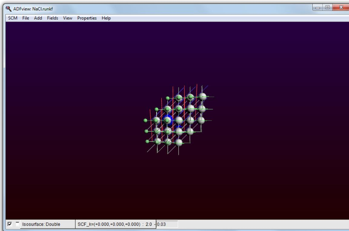
If you rotate it a bit and toggle the isosurface on and off (with the check box in front of it), you can convince yourself that this orbital is located around the small atom, which is the Chlorine.
