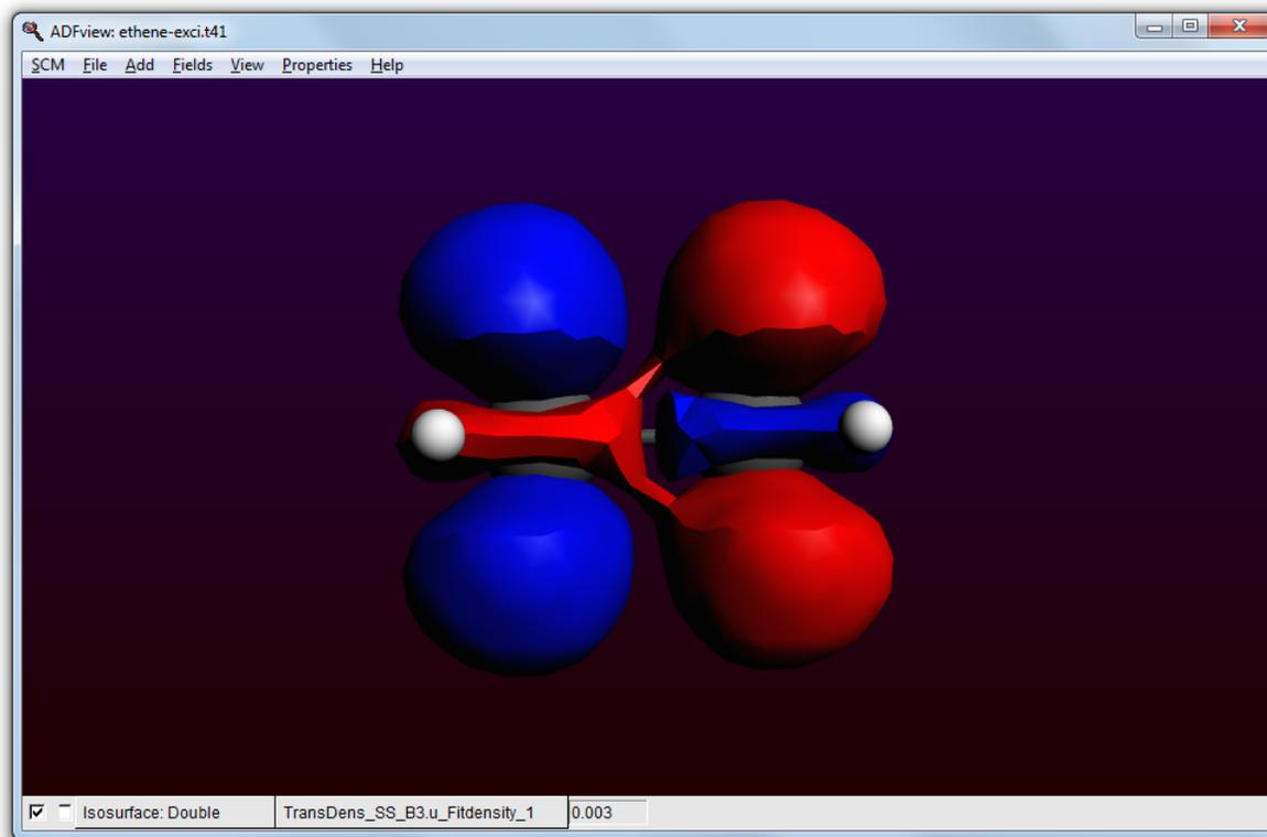
The resolution is rather coarse, you can use interpolation to get a better picture. Changing the grid has no effect in this case as you are visualizing a .t41 file, which is just data on a grid (in binary form).
