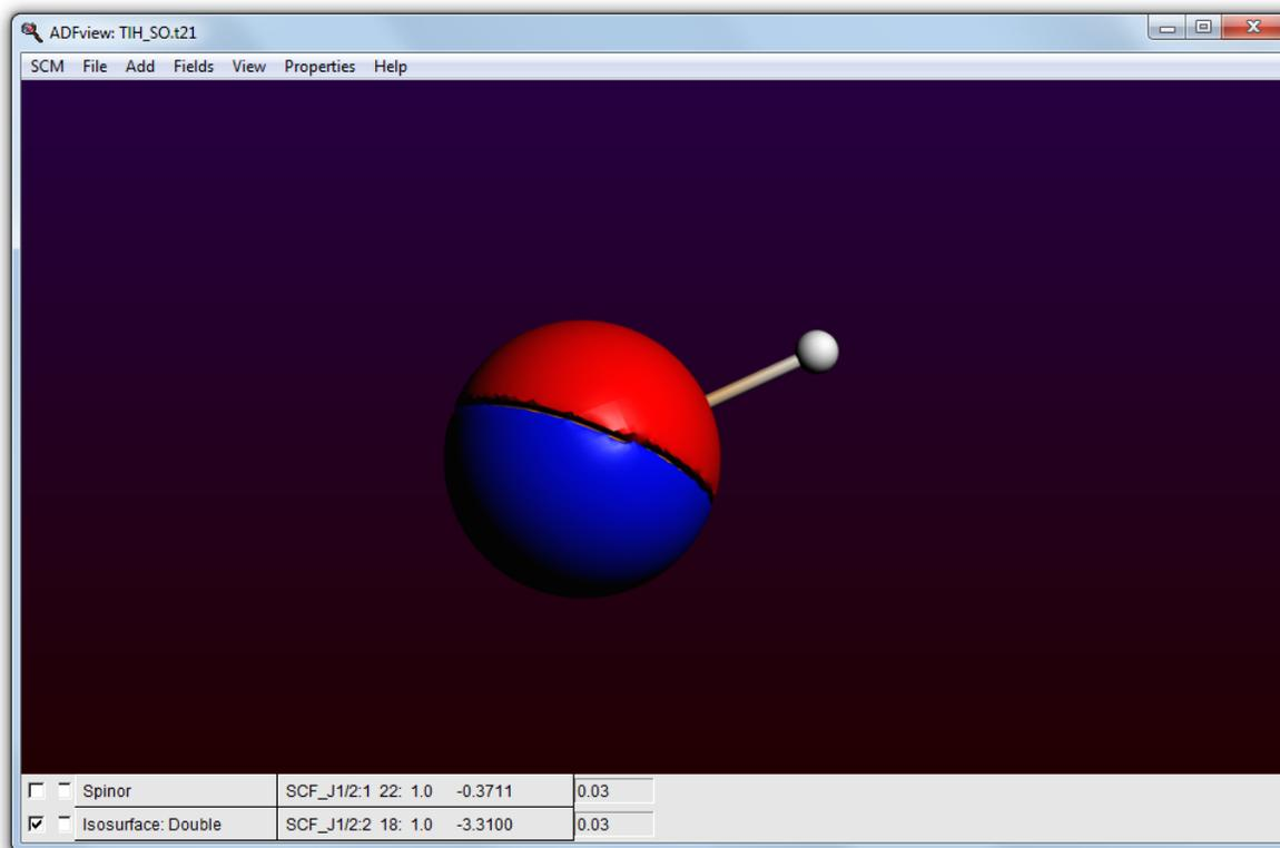
This spinor  $18j_{1/2}$  is almost a pure  $5p_{1/2}$  TI spinor. A  $p_{1/2}$  atomic orbital has a spherical atomic density, but a spin magnetization density which is not the same in each point in space.
