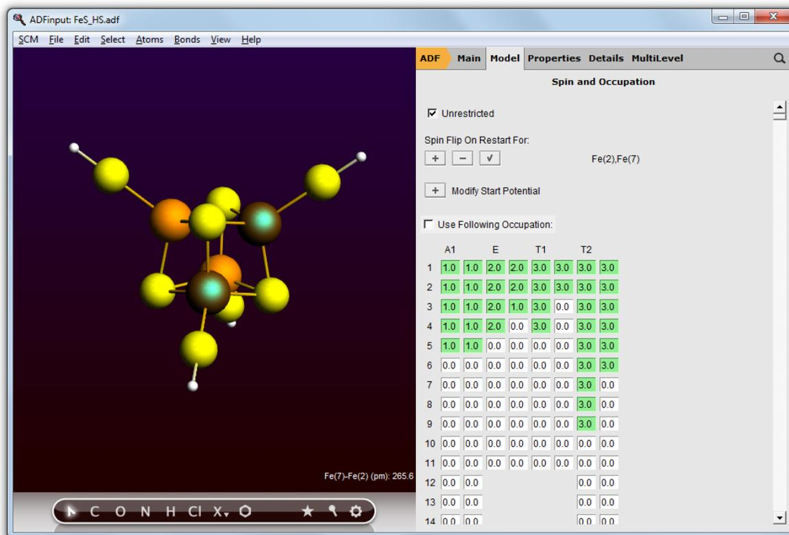
To achieve the desired BS solution, the SpinFlip procedure should be applied to 2 out of 4 Fe sites of Fe<sub>4</sub>S<sub>4</sub>. In the above example, we selected sites Fe(2) and Fe(7). This will instruct SpinFlip algorithm to interchange  $\alpha$  ( $\uparrow$ ) and  $\beta$  ( $\downarrow$ ) electron densities associated with these two Fe sites when the job will be restarted, changing the HS 4 $\uparrow$ :0 $\downarrow$  spin state to the BS 2 $\uparrow$ :2 $\downarrow$  spin state.
