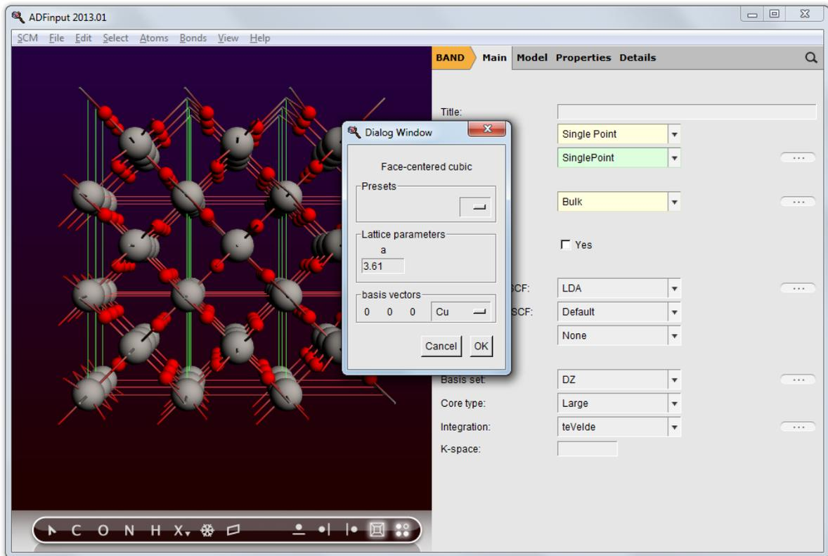
Press "OK" to generate the Cu lattice
