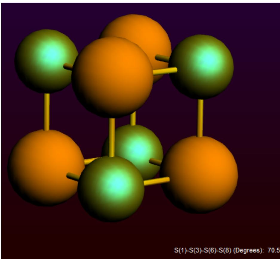
Now you should see the Fe<sub>4</sub>S<sub>4</sub> cubane in the structure drawing area of ADFinput. The proper coordination to Fe atoms is important in modeling their electronic structure. In proteins, iron-sulfur cubanes are coordinated by cysteine ligands to the Fe sites. Here, we will model these four cysteines by <sup>-</sup>SH ligands. The procedure to add these ligands is described below.
