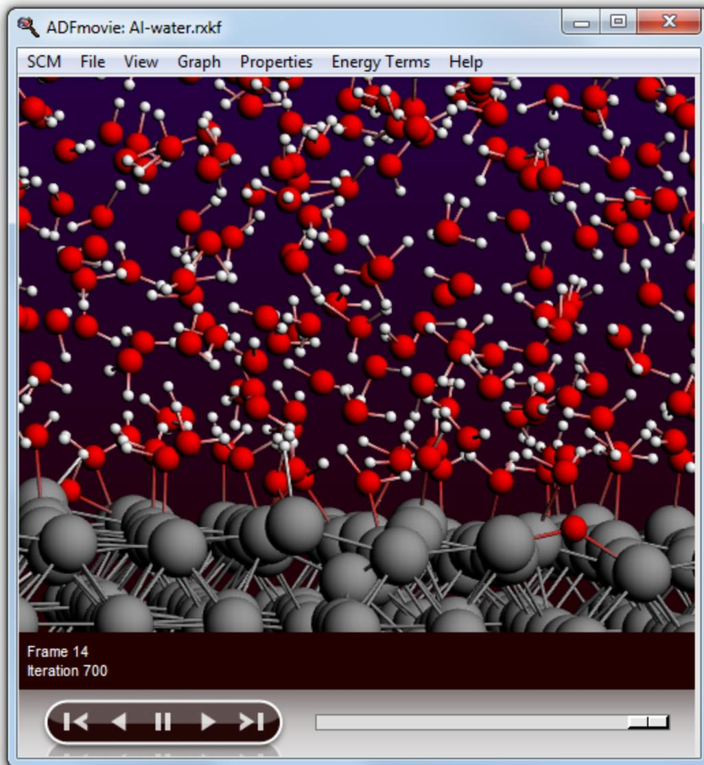
If you look around, you will most likely see many water molecules attaching to the aluminum surface. After some time, you might also see hydrogen atoms distracted from the water molecules, which are now moving around the surface on their own.
