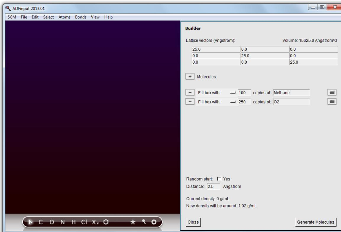
At the bottom of the Builder panel you can see that the current density is zero. The new density, after adding methane and oxygen, will be around 1 g/mL, which is obviously very high for this mixture. For this tutorial that is fine as it means things will happen faster.
